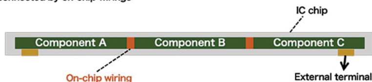
Conventional semiconductor integrated circuits (IC chip): Circuits are connected by on-chip wirings
