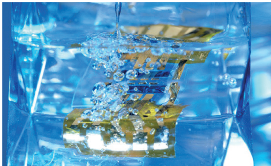
Ultra-thin organic solar cells that can be operated underwater for long periods of time.
