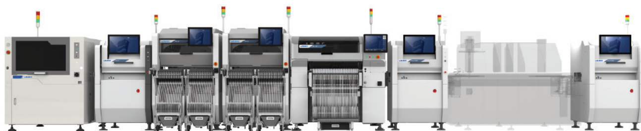
The latest SMT line centered on the High-Speed Compact Modular Mounter "RX-8"
