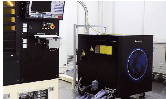
Photo 1: Blue laser processing machine under development as a next-generation processing machine.
