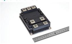
New 3.3kV/400A and 3.3kV/200A versions of Mitsubishi Electric's SBD-embedded SiC-MOSFET module, together with the existing 3.3kV/800A, comprise the new Unifull™ series.
