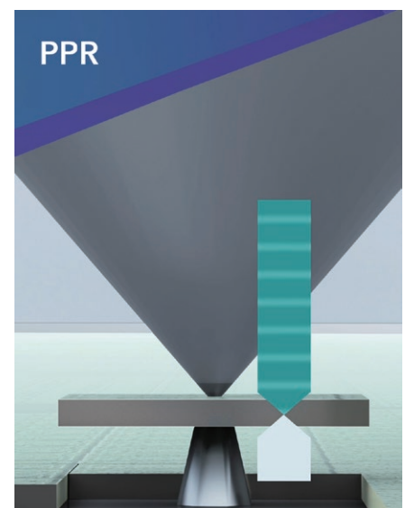
Impact absorbed by avoiding overlapping forces as the chip is pushed up
